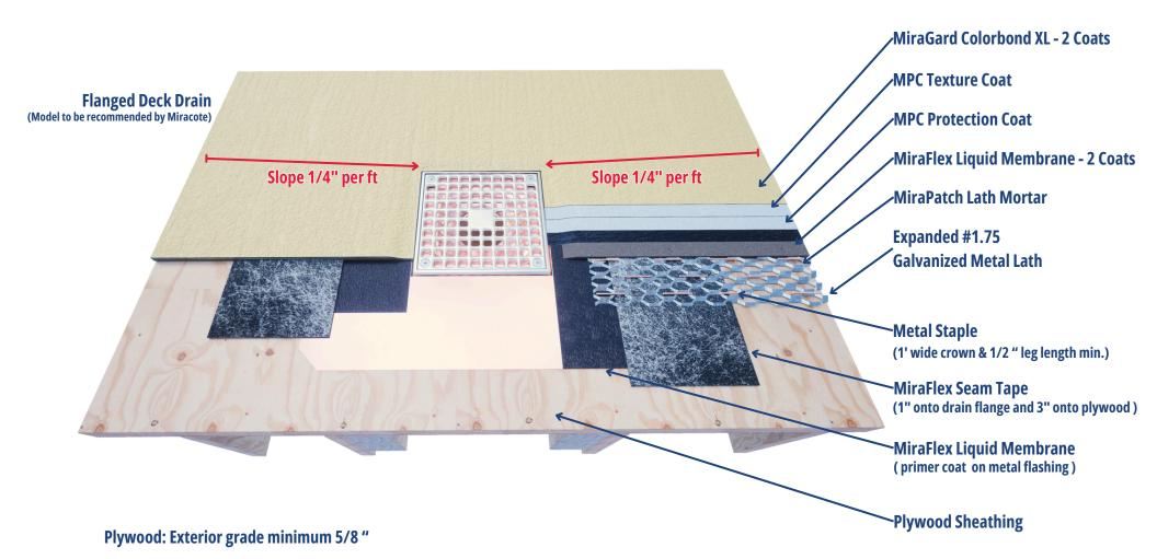
One-piece flanged deck drain with full perimeter blocking and securing over MiraFlex Hybrid Sealant
