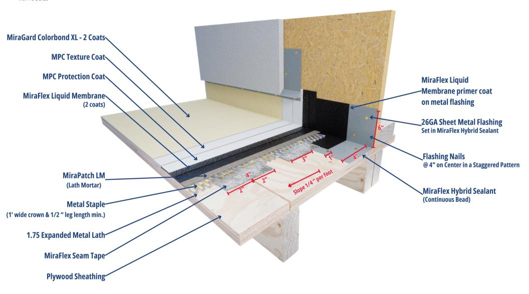
Plywood: Exterior grade minimum 5/8 " sheathing fully blocked, glued and screwed, no deflection.
