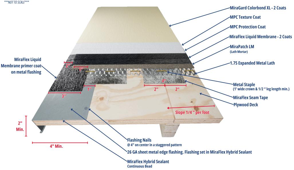
Plywood: Exterior grade minimum 5/8 " sheathing fully blocked, glued and screwed, no deflection.
