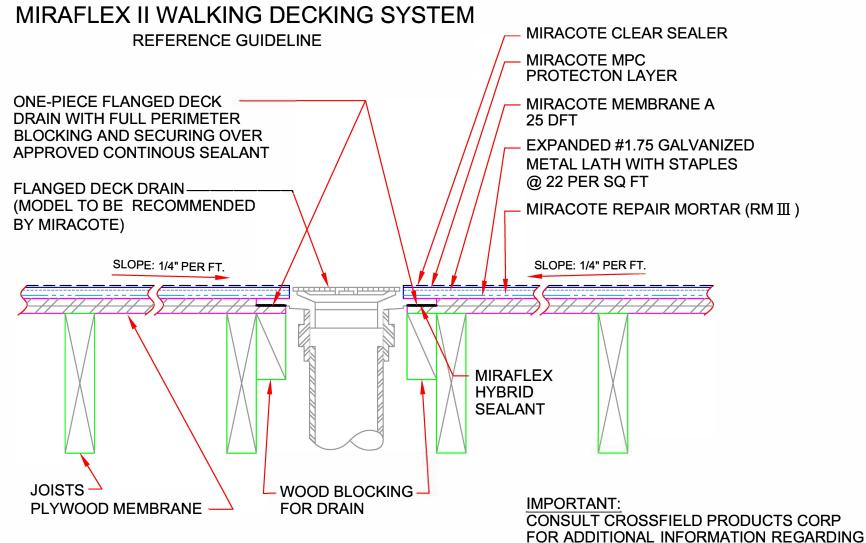
NOTE: PRIOR TO FASTENING DRAIN FLANGE TO PLYWOOD AND WOOD BLOCKING-SET FLANGE INTO WET MIRAFLEX HYBRID SEALANT OR OTHER APPROVED EQUAL —NO DEFLECTION.
