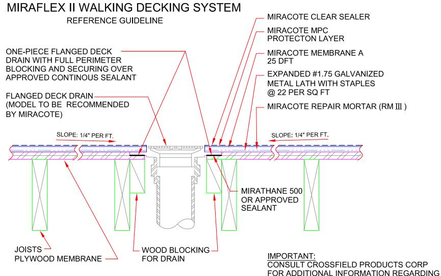
NOTE: PRIOR TO FASTENING DRAIN FLANGE TO PLYWOOD AND WOOD BLOCKING-SET FLANGE INTO WET MIRATHANE 500 OR OTHER APPROVED SEALANT NO DEFLECTION.
