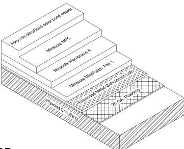
Plywood Substrate at Wood or Metal Stud Wall Detail #3B
